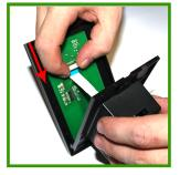
2.) Push down on both sides of the black plastic quick connector and remove the connecting wire.
