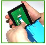
4.) Re-insert the connecting wire with the blue side facing up. See further steps for more details.
