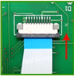
6.) Insert the wire into the connector and pinch the black plastic closed as seen in the photo above.
