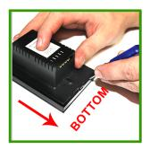
1.) Using a small flat head screwdriver gently pop out the bottom of the touch panel.
