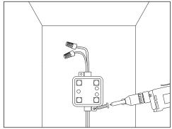
FASTENERS: If desired, modules can be secured with #4 X 1/2" metal screws.
