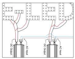
Using predetermined layout and LED placement from step 1, divide channels into sections and distribute each section to corresponding power supplies.
